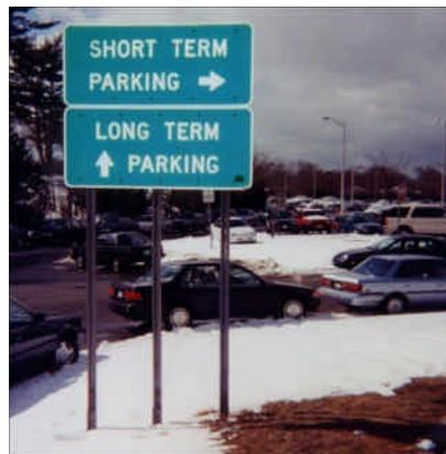
Figure 2: This sign at the Central Islip station on the LIRR is an example of a way to separate kiss-and-ride traffic from park and ride traffic. Unfortunately, due to illegal parking, if one follows the arrow for short-term parking it leads to occupied curbside space.
